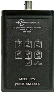
The S250 simulates pH or ORP signals that would normally be generated by the electrode. It can be used for troubleshooting to confirm that any pH or ORP meter is functioning correctly. This can also be used to certify a device prior to installation or batch. The S250 has outputs for 4, 7 and 10 pH and +700m and -700mV for ORP. It also has a High Meg ohm impedance option that is critical for simulating the high impedance of the pH glass and testing the amplification circuitry.
