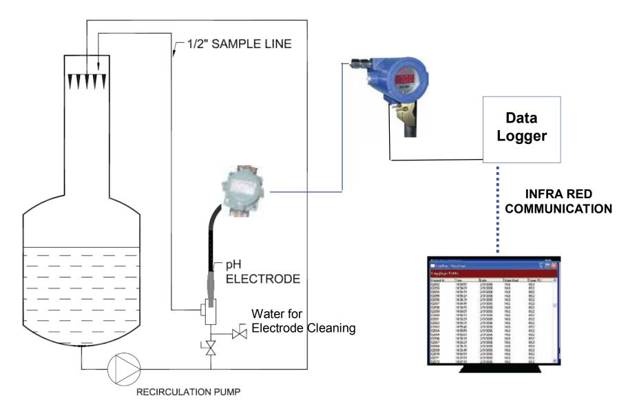
The scrubber system comprises a pH Electrode in Chemical resistant RYTON™ body, a pH Transmitter located close to the electrode, a pH indicator and a Battery operated Data Logger to record the Scrubber pH readings with a Time stamp. The Data logger is a convenient stand alone Battery operated unit with 16,000 readings memory. The data logger is equipped with IR communication for transfer of logged data to any PC.
